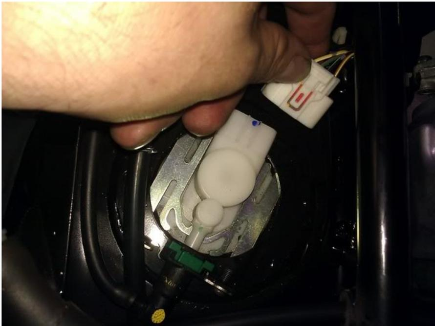
then relieve the fuel pressure. turn ignition on and press the starter for 5 seconds. After that, remove the fuel line, fuel line clamp bolt, and th
