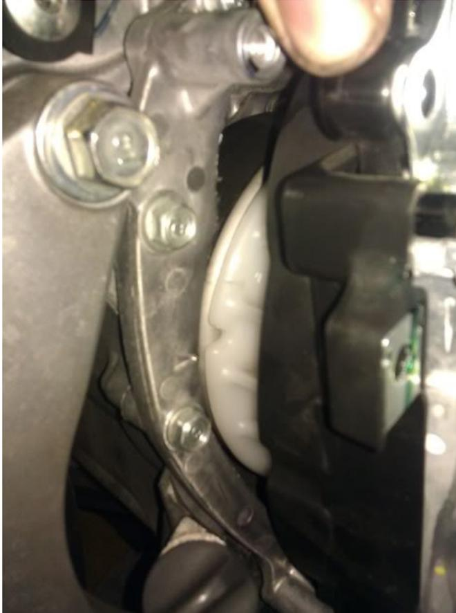
turn the crankshaft COUNTER CLOCKWISE until the index mark and the cutout on the fan line up as pictured above, test to see if there is slack giving it a wiggle
