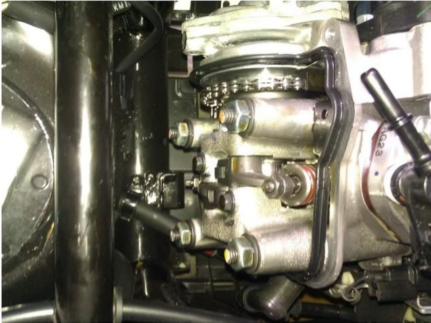
then remove 3 bolts on the left cover exposing the crankshaft
