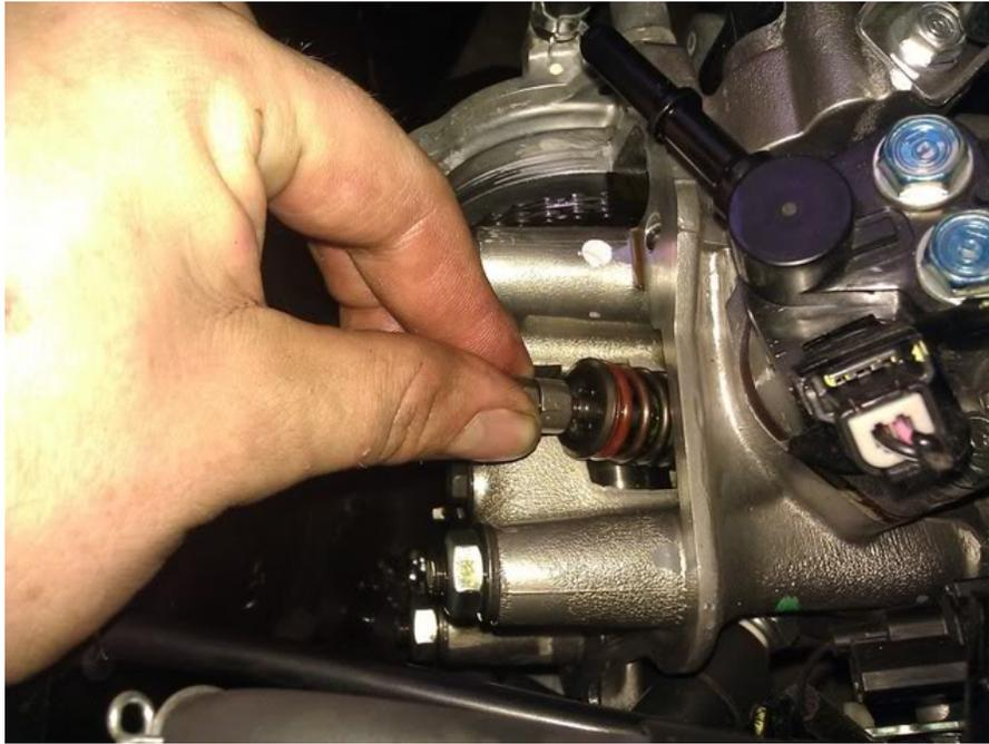
if it feels like its not moving then you will need to spin the crankshaft a full 360 degrees to be at top dead center. Verify that the index mark a again, and verify that the index line and the punch mark on the camshaft line up pictured below:
