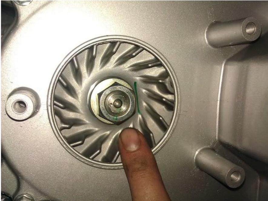
Remove the right side radiator cover (3 bolts) and remove the 4 bolts holding the radiator on to expose the fan. Do not disconnect any hoses
