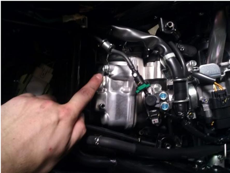
pull up on the green tab to remove: use a rag to catch excess fuel
